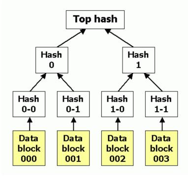
In a merkle tree, hashes propagate upward in a way that if data is altered on the bottom of the tree, the hashes above that data will be changed. For example from the diagram above, if the data in "Data block 000" is changed then "Hash 0-0" will be changed, as will "Hash 0," as will the "Top Hash." An upward ripple effect can be observed from the changing of data at the bottom of the tree.
